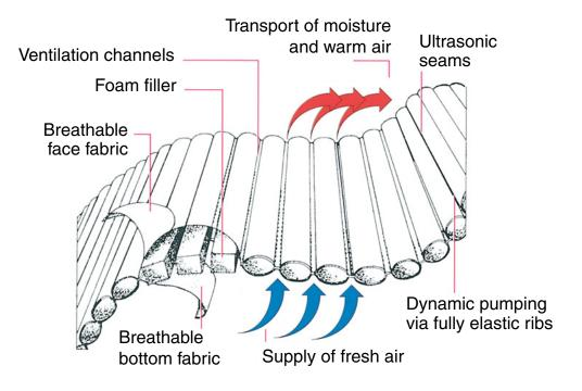
1. pneumolastic is a patented, ultrasonically produced, textile, bonded material.
